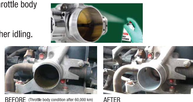
BEFORE (Throttle body condition after 60,000 km)
