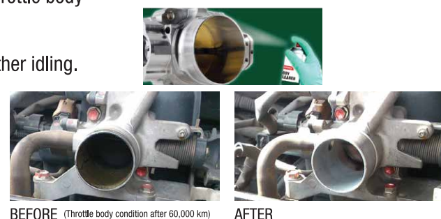
BEFORE (Throttle body condition after 60,000 km)
