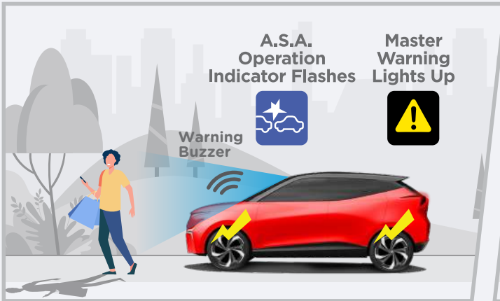
Warning buzzer + primary brake (weak)
