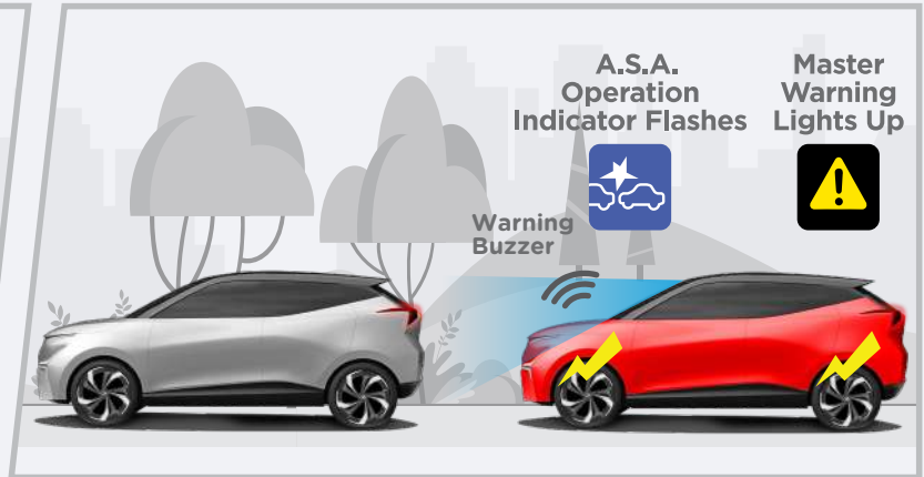
Warning buzzer + primary brake (weak)
