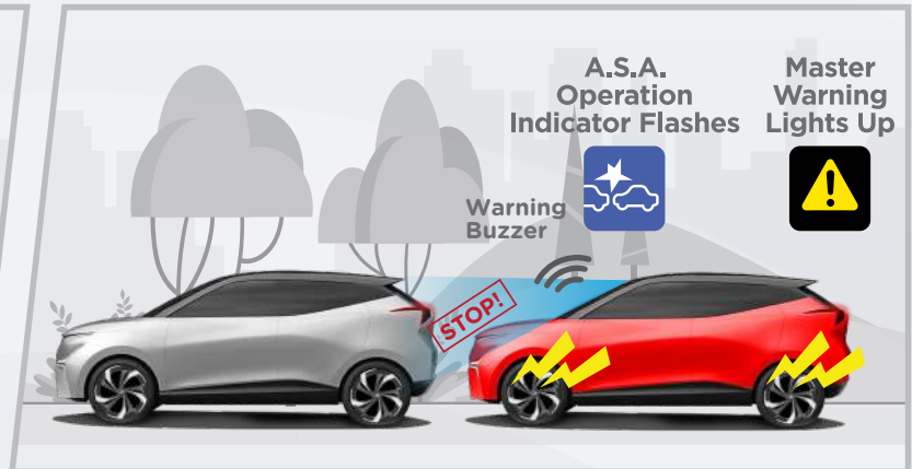
Warning buzzer + secondary brake (strong)
