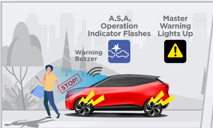
Warning buzzer + secondary brake (strong)
