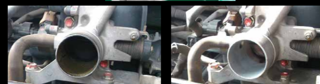
BEFORE (Throttle body condition after 60,000 km) AFTER
