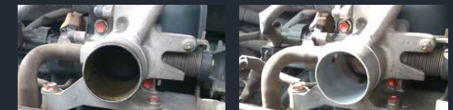
BEFORE (Throttle body condition after 60,000 km)
