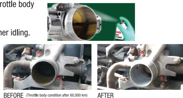
BEFORE (Throttle body condition after 60,000 km)
