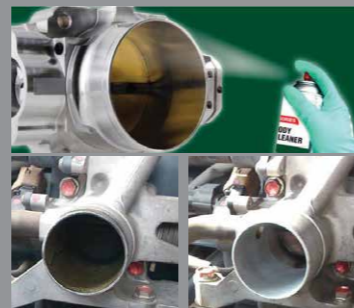
BEFORE AFTER (Throttle body condition after 60,000 km)
