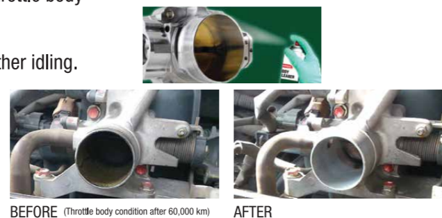
BEFORE (Throttle body condition after 60,000 km)
