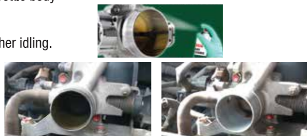
BEFORE (Throttle body condition after 60,000 km) AFTER
