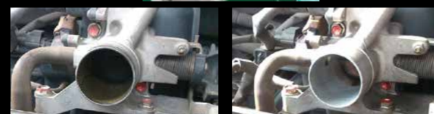
BEFORE (Throttle body condition after 60,000 km) AFTER
