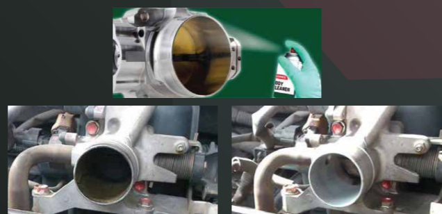
BEFORE (Throttle body condition after 60,000 km) AFTER
